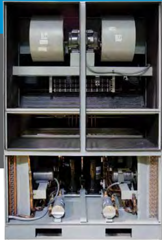
Rear View (From outside the conditioned area). Note the redundant compressors and blowers, as well as optional electric heat and filter dryers.
